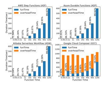
Fig. 8. The performance of various levels of function complexity in sequence workflow.
