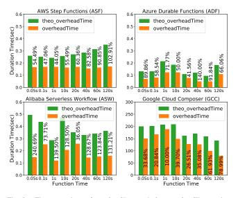
Fig. 9. The comparison of *overheadTime* and *theo\_overheadTime* under various levels of function complexity in parallel workflow.
