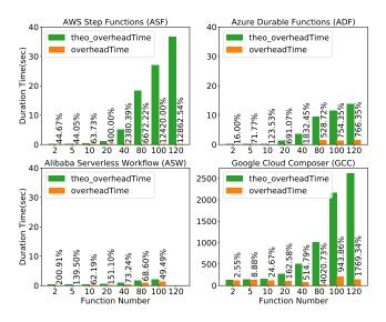
Fig. 5. The comparison of *overheadTime* and *theo\_overheadTime* under various levels of activity complexity in parallel workflow.
